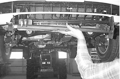
3. Install cross member with three 3/8" x 1-1/4" hex bolts, lockwashers and hex nuts on each side.
